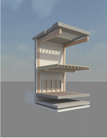
Here it is possible to see how the wood construction is exposed in various ways through the building.
